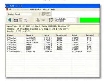
Communications software between Aquamax KFVolumetric and PC
